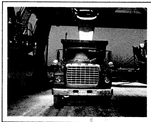
An electronic weigh hopper records each load and registers total weight discharged.
